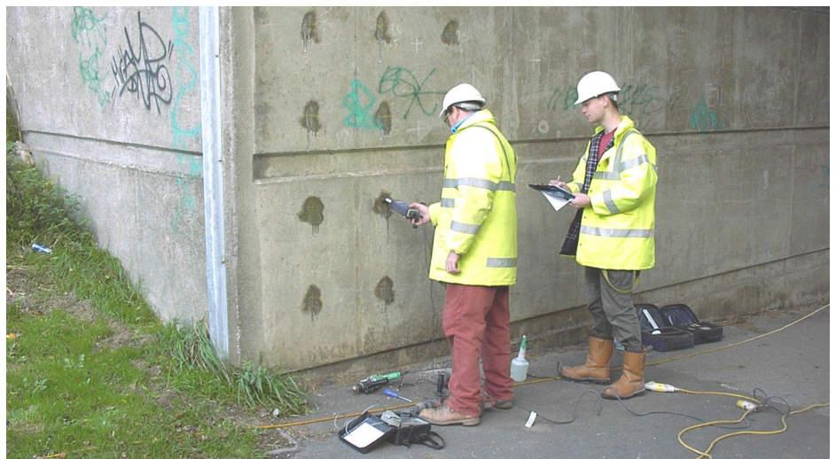
Half cell potential testing by in-house UKAS accredited personnel.
